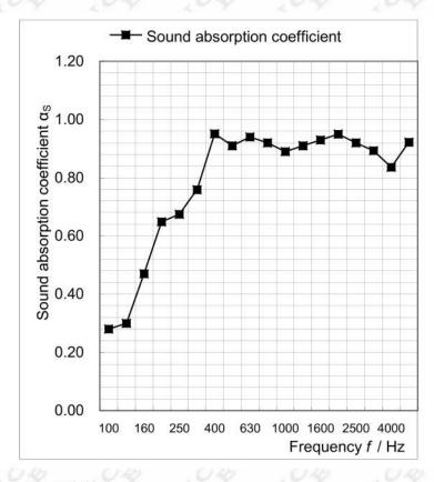
α<sub>S</sub> Sound absorption coefficient according to EN ISO 354
