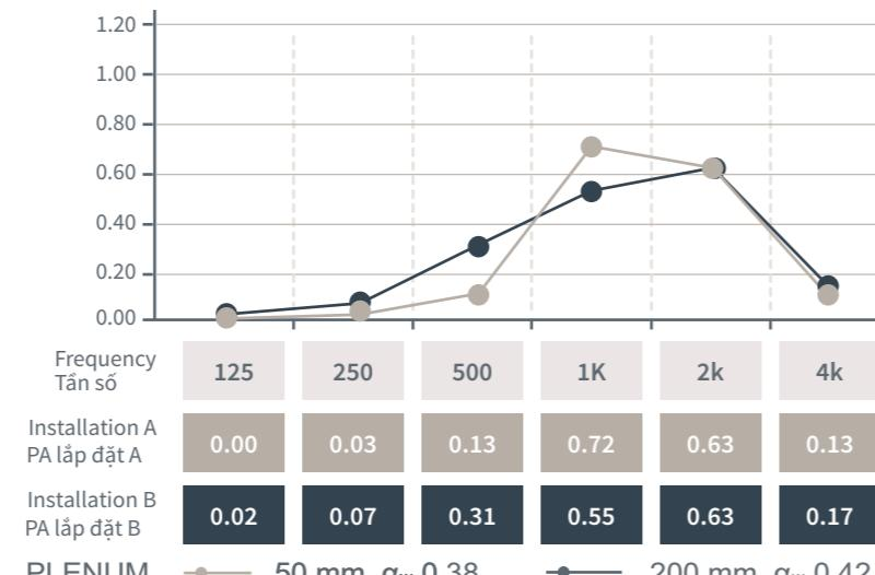
● Installation A : 50mm Remak® rockwool insulation
