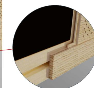
10mm solid skirting pinned and glue fixed to wall battens.
