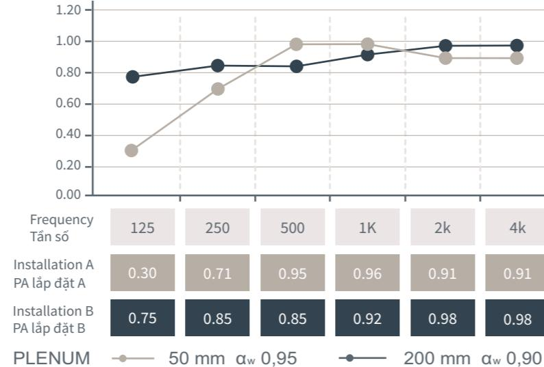
**Installation system:** various installation possibilities over wooden battens or metal profiles, with clips or directly attached to the structure. In order to obtain an optimum absorption coefficient, it is necessary to leave a space of at least 30 mm between the back of the panels and the wall, filled with Remak® Rockwool fiber with a density between 40 and 50 kg/m<sup>3</sup>.
