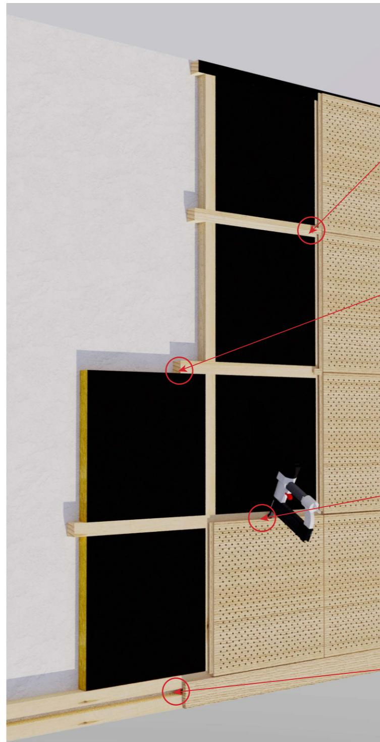
Loose tongue with specified face finish, creating 6mm shadow gap between tiles. These dimensions can be adjusted to your desired specifications.
