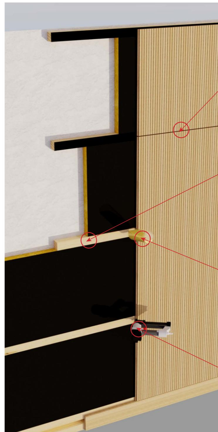
Allow a 3-5mm shadow gap at end of planks. For best results, use the aligned style as shown and paint battens black where visible.
