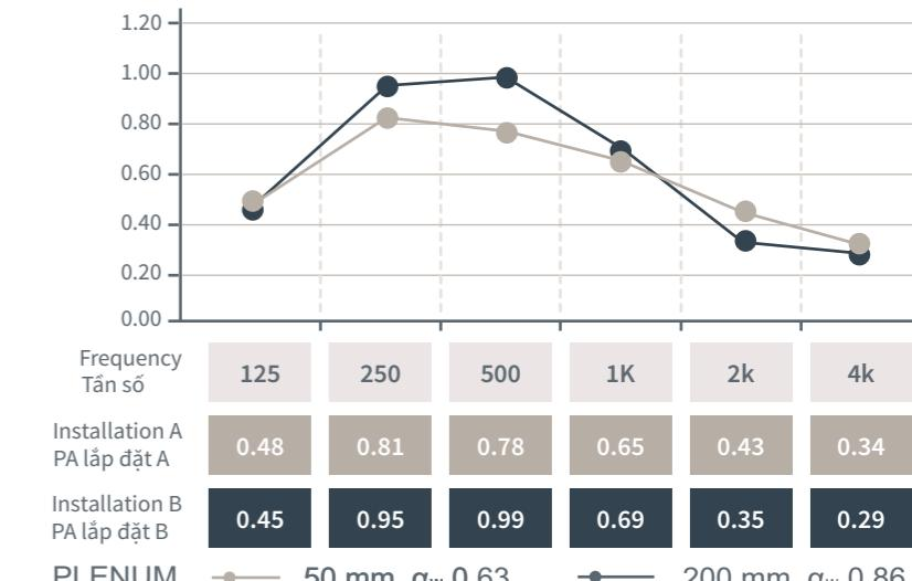
● Installation A : 50mm Remak® rockwool insulation
