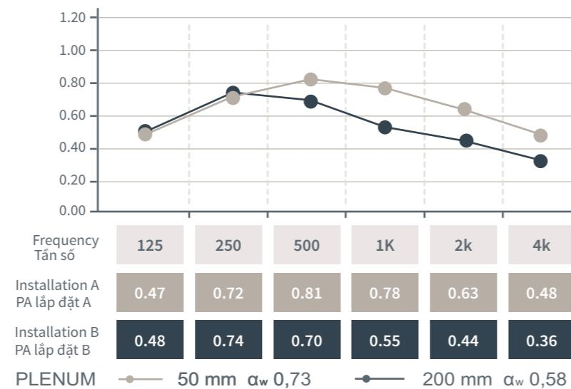
**Installation system:** various installation possibilities over wooden battens or metal profiles, with clips or directly attached to the structure. In order to obtain an optimum absorption coefficient, it is necessary to leave a space of at least 30 mm between the back of the panels and the wall or ceiling, filled with Remak® Rockwool fiber with a density between 40 and 50 kg/m<sup>3</sup>.
