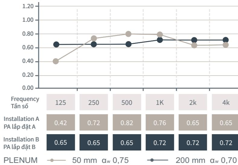
● Installation A : 50mm Remak® rockwool insulation
