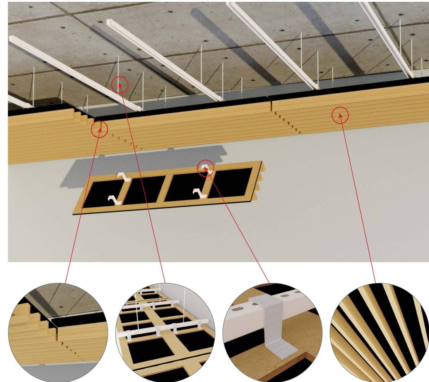
Allow a 10-50mm shadow gap between modules and 25-50mm at perimeter.
