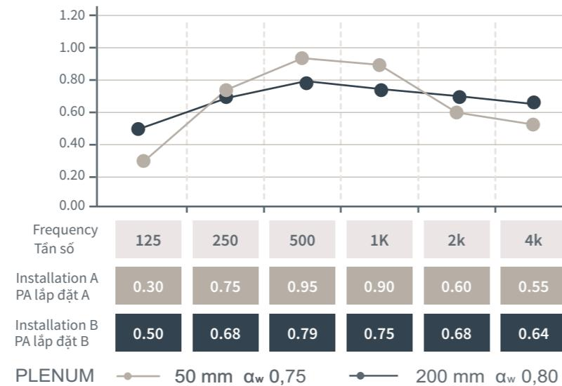
**Installation system:** various installation possibilities over wooden battens or metal profiles, with clips or directly attached to the structure. In order to obtain an optimum absorption coefficient, it is necessary to leave a space of at least 30 mm between the back of the panels and the wall or ceiling, filled with Remak® Rockwool fiber with a density between 40 and 50 kg/m<sup>3</sup>.
